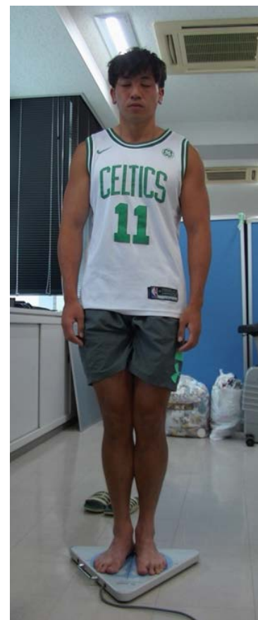
Figure 2: Measurement of static postural stability using a center-of-gravity sway meter.
