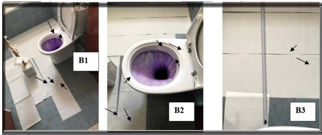
Figure 2b: Dye added to the cistern (B1, B2 & B3) drops 40 cm away from the toilet (B3)
