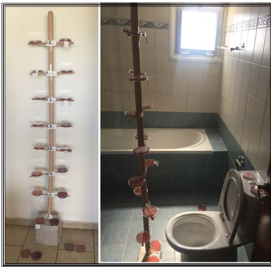
Figure 1: The plate-tree after construction and in position in toilet 1 (T1) after flushing
