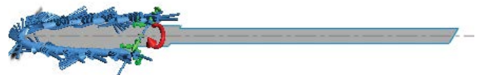
Figure 10: Axial (longitudinal) planes for the geometric model of the dental bur, after applying the simplifying assumptions.
