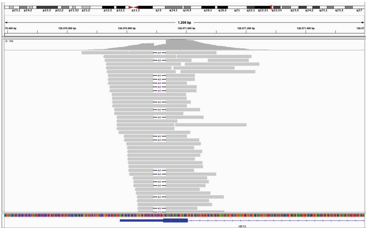
Figure 2: The deletion involves the loss of 31 nucleotides in the 5'UTR region and 10 nucleotides in the upstream open reading frame (NT: ATGAAGCGCC). The deletion removes a regulatory sequence that consequently leads to increased expression of the HEY2 protein (IGV software).
